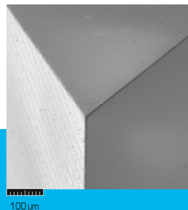
DLC3 coated endmill under scanning electron microscope:
