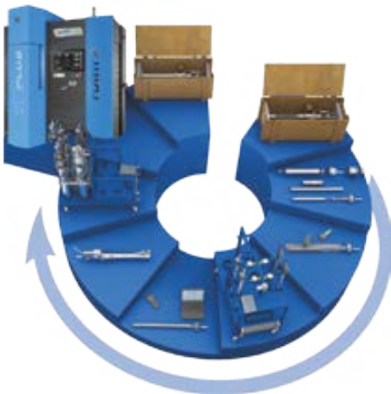
Process of cathode exchange
